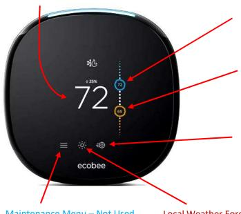
Touch and drag blue circle to change the temperature at which the A/C comes on
